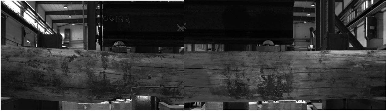
Figure 5. Set-up for destructive four-point bending test with typical failure in bending: fibre splitting.
