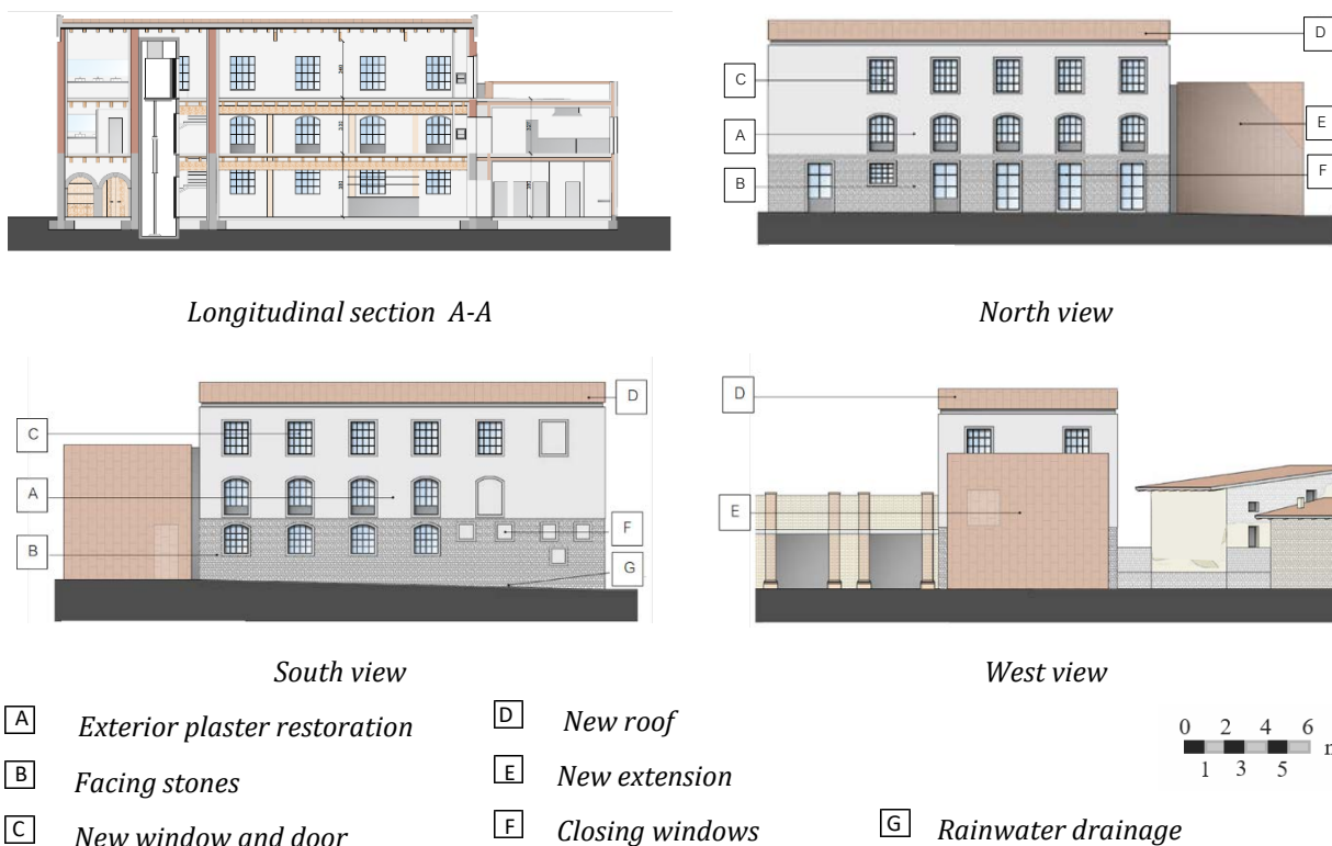
Figure 6. Project elevation views
