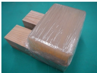
Figure 1. The decay source unit
