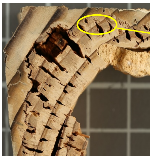
Figure 9. Catastrophic damage by wet-brown-rot: top-centre image – white fruiting body indicates most probably Rhodonia placenta (under the leaking roof window); bottom images – micrographs at different magnifications of decayed wood tissue in close to surface zone with lots of cracks.
