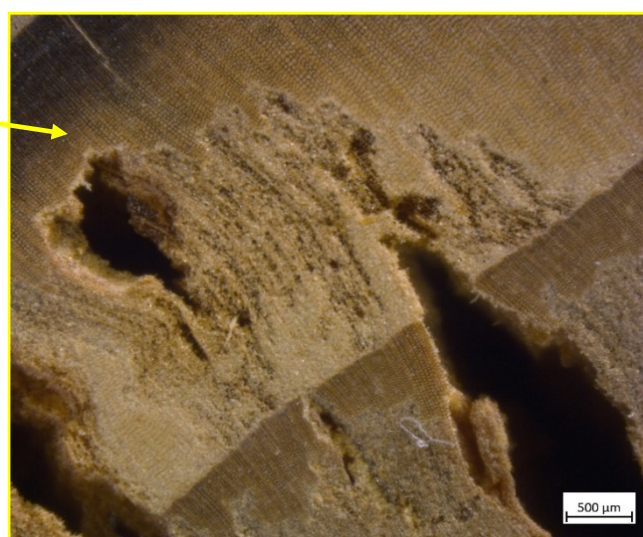
Figure 9. Catastrophic damage by wet-brown-rot: top-centre image – white fruiting body indicates most probably Rhodonia placenta (under the leaking roof window); bottom images – micrographs at different magnifications of decayed wood tissue in close to surface zone with lots of cracks.
