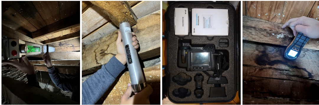
Figure 7. (a) Controlled perforation test; (b) Surface hardness test; (c) Thermographic camera; (d) Water content measurement with hygrometer
